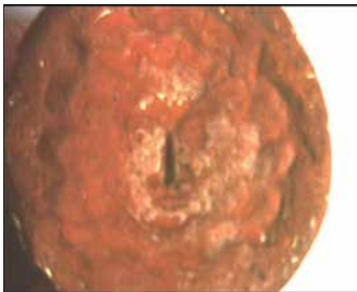
Figure 40.11. A clay mould for casting applications of copper alloy depicting a Medusa (by D. Ratković, 2011).
